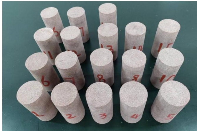
Fig. 1. Red sandstone specimens processed into standard cylinders (50 mm × 100 mm) (He et al. , 2026).
