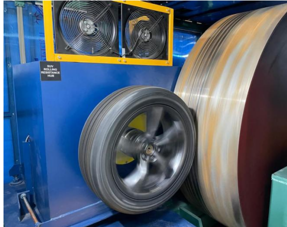
Fig. 1. Schematic of the experimental setup used for RR measurements in accordance with ISO 28580.
