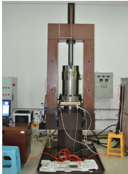
Fig. 1. TFD-2000 electro-hydraulic servo rock triaxial testing machine.
