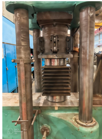
Fig. 1. Test bench set to measure spring characteristics.
