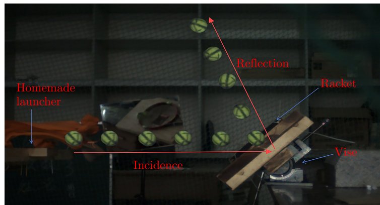
Fig. 1. Superimposition of multiple images of actual tennis incidence and rebound.
