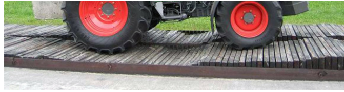
Fig. 17. ISO 5008, rougher road course in reality.
