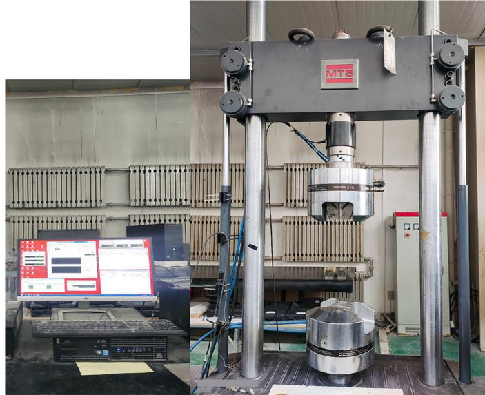
Fig. 2. MTS-793 rock mechanics testing machine.
