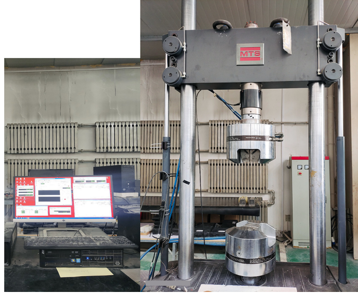
Fig. 2. MTS-793 rock mechanics testing machine.
