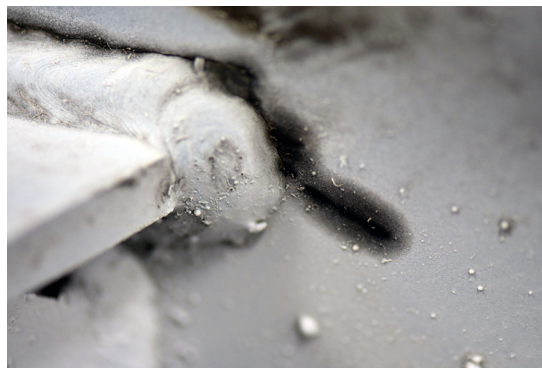
Fig. 9. Hair cracks in a component made of high-strength steel (S700MC) using dye-penetrant technique after 2 \times 10^6 cycles.
