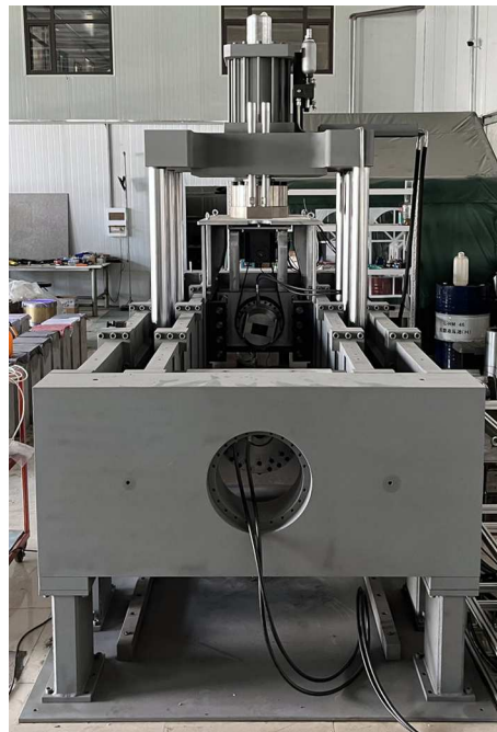
Fig. 5. The RTR-3122 full-scale anchorage performance tester
