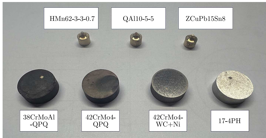
Fig. 2. Representation of slipper/eccentric cam pin-on-disc tribopairs
