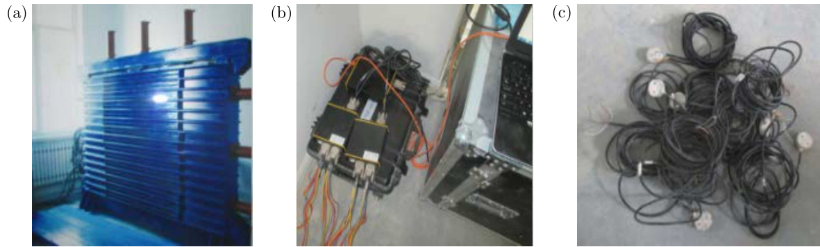
Fig. 2. Schematic diagram of the testing device: (a) test bracket, (b) strain analyzer, (c) pressure cell
