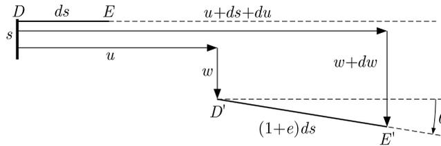
Fig. 2. Schematic of a beam displacements
