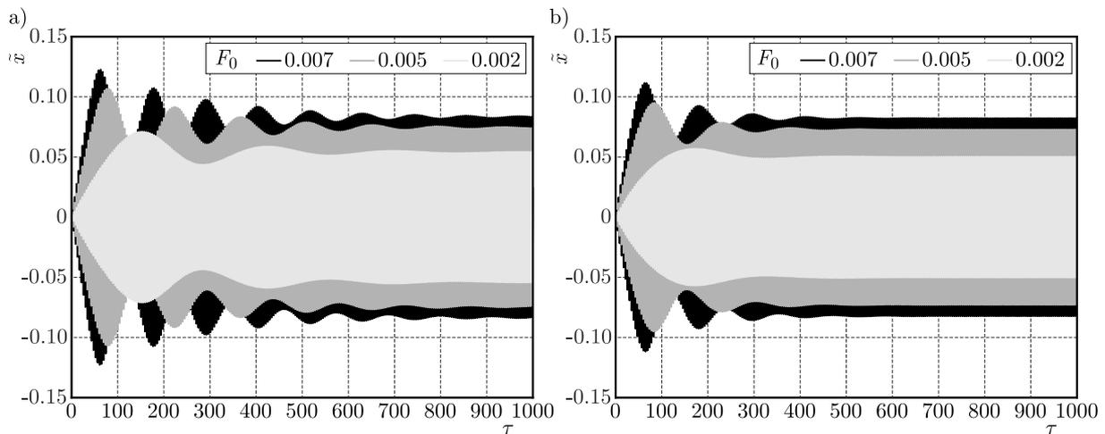
Fig. 10. Nonlinear beam response, harmonic excitation,  $\gamma = 0.5$ : (a)  $\tilde{\mu}_\gamma = 0.008$ , (b)  $\tilde{\mu}_\gamma = 0.016$
