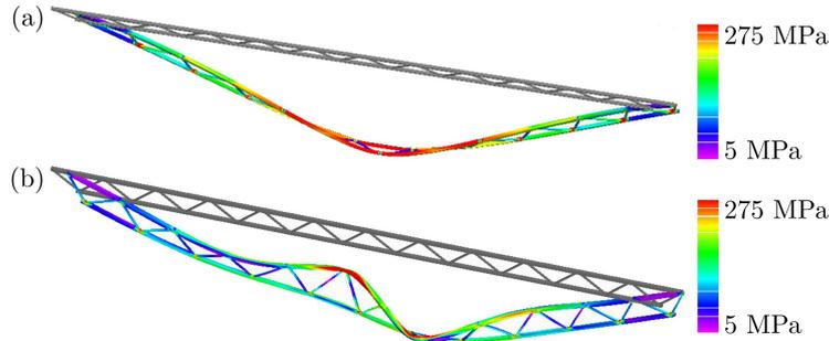
Fig. 8. The deformation and the stress state (HMH hypothesis, top surface of the shell model element) at the limit load for the braced truss  $k = 100 \text{ kN/m}$ ,  $k_{rot} = 5 \text{ kNm/deg}$  with an imperfection in the form of: (a) arch curvature, (b) buckling mode
