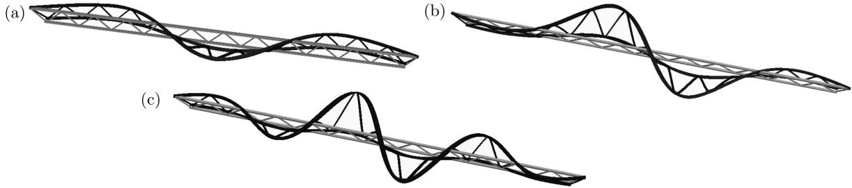
Fig. 5. Buckling modes for the truss (beam and shell models) with braces of stiffness: (a)  $k = 100$  kN/m or  $k_1 = 100$  kN/m,  $k_2 = 112.5$  kN/m,  $k_3 = 180$  kN/m and  $k_{rot} = 0$  kNm/deg, (b)  $k_1 = 100$  kN/m,  $k_2 = 112.5$  kN/m,  $k_3 = 180$  kN/m and  $k_{rot} = 5$  kNm/deg or  $k_{rot} = 10^6$  kNm/deg, (c)  $k = 10^6$  kN/m or  $k = 10^6$  kN/m and  $k_{rot} = 10^6$  kNm/deg
