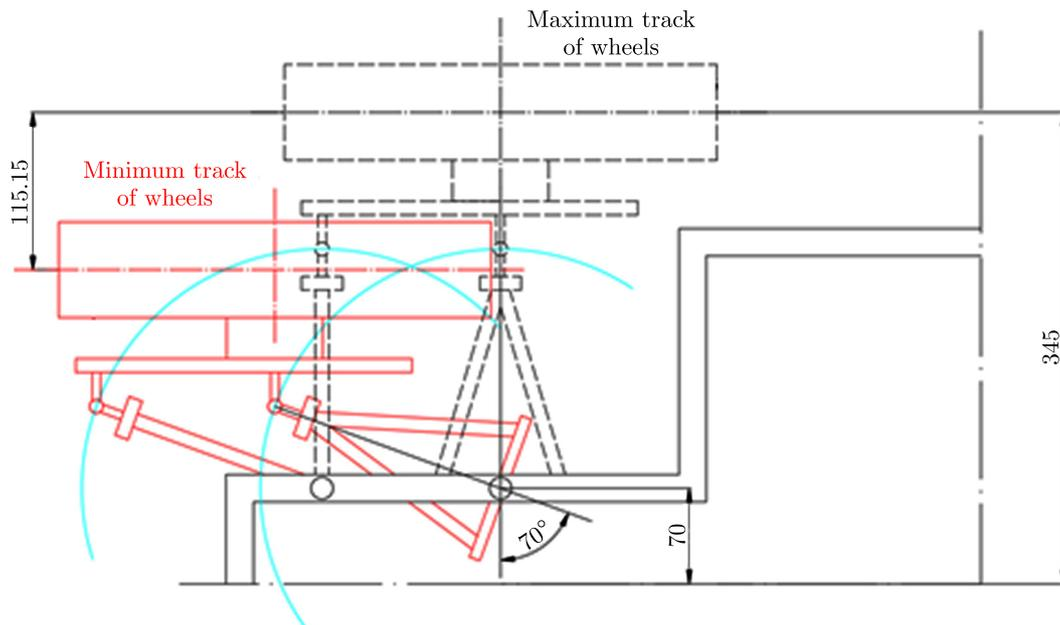
Fig. 4. Scheme presenting the working principle of the mechanism changing the track of wheels
