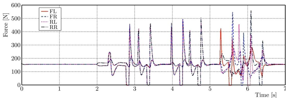
**Fig. 9.** Vertical ground reaction force on each wheel (FL, FR – front left and right, RL, RR – rear left and right) for simulation 2 while driving over the 3 step obstacles with the controlled damping coefficient
