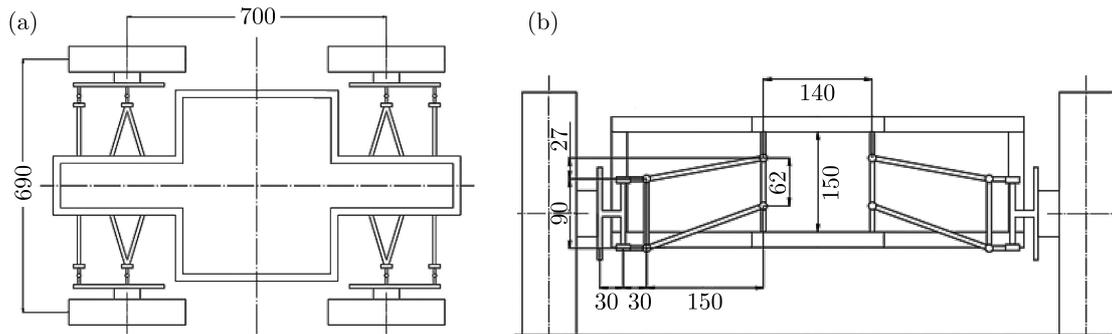
Fig. 3. Designed dimensions (in mm) indicated in: (a) an overall scheme of the mobile platform, (b) a scheme with details of the suspension system
