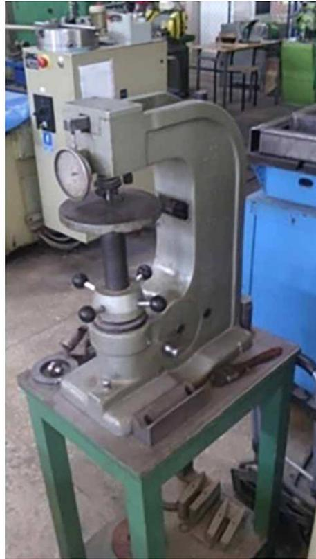
Fig. 7. Hardness tester PRL 610
