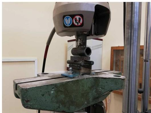
Fig. 5. Bending resistance test
