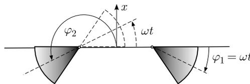
Fig. 3. System of phase angles of vibrators in the synchronous running state
