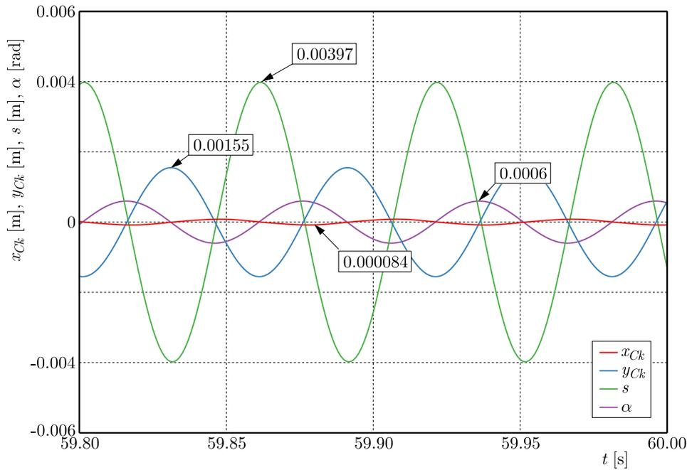
Fig. 4. Pathways of generalized coordinates in the steady state obtained on the basis of dynamic equations (2.6)-(2.11)
