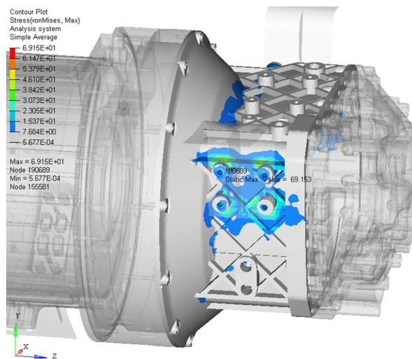
Fig. 7. Stress cloud for working condition 9
