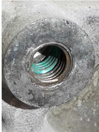
Fig. 2. Support hole thread the gearbox case
