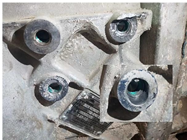
Fig. 1. Rupture position of the support hole
