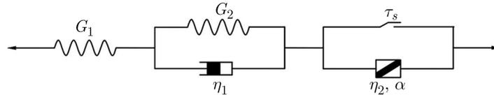
Fig. 8. Schematic of the nonlinear fractional Burgers model
