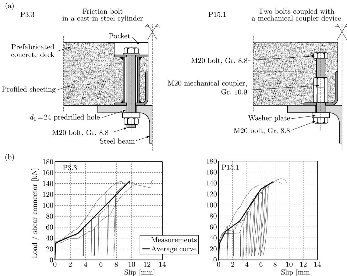
Fig. 3. Investigated demountable shear connectors: (a) section of System P3.3 and System P15.1, (b) load-slip curves from push tests
