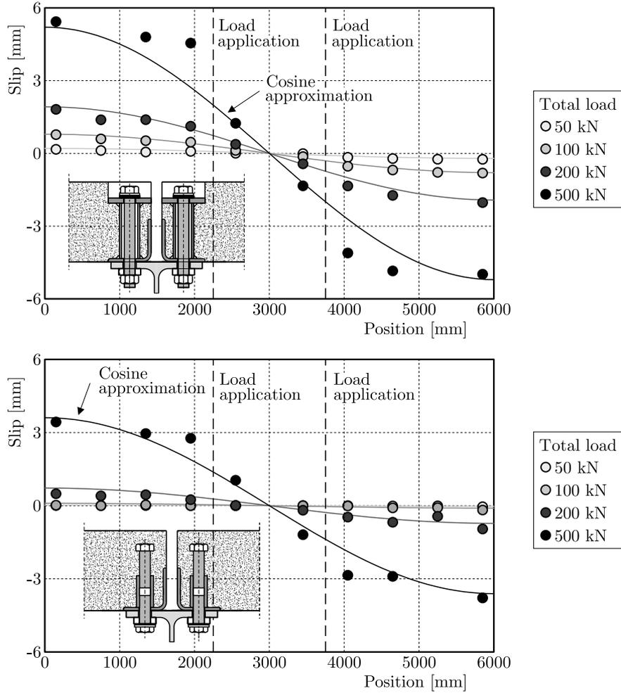
Fig. 4. Slip distribution measured from beam tests (6 m span beam)
