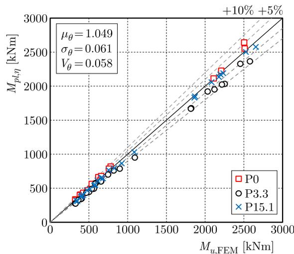
Fig. 8. Comparison of the moment resistance obtained from the FEA and simplified algorithm
