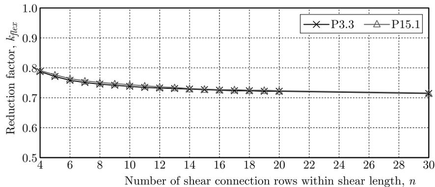
Fig. 5. The relationship of the reduction factor  $k_{flex}$  and the number of shear connector rows  $n$
