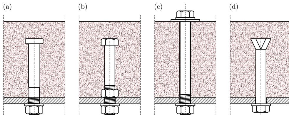
Fig. 1. Bolted shear connectors overview: (a) threaded studs, (b) encased bolts, (c) through bolts, (d) anchor bolts and blind bolts
