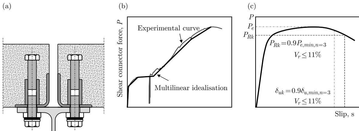
Fig. 2. An example of a demountable shear connector: (a) illustration image, (b) multilinear load-slip curve, and (c) load-slip curve implied in Eurocode 4 for welded studs (CEN, 2018)
