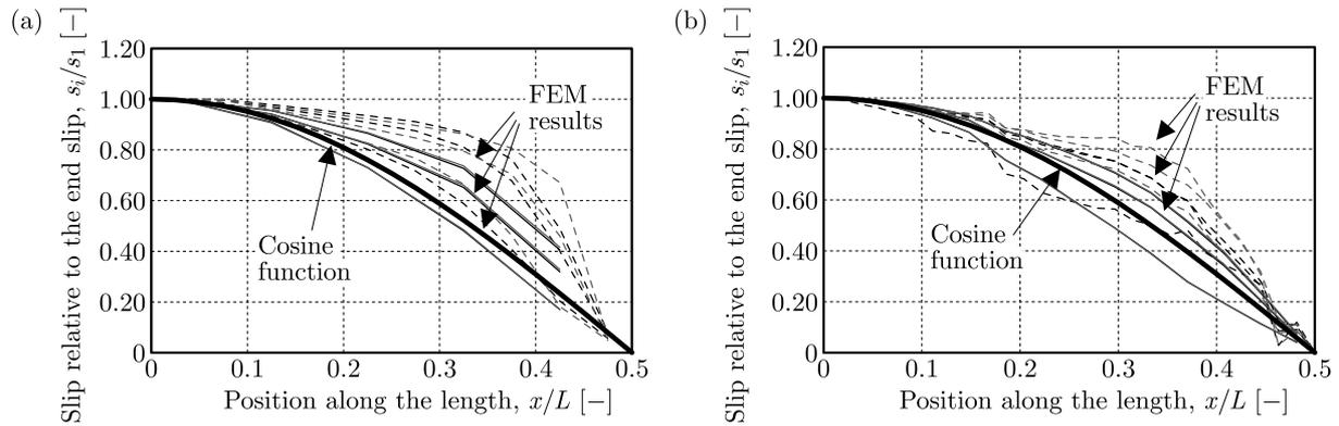
Fig. 7. Relative slip distributions in comparison with a cosine function: (a) results of 6 m demountable composite beams, (b) results of 16.2 m demountable composite beams
