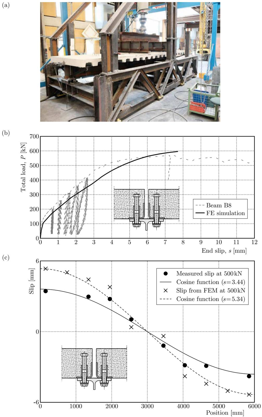
Fig. 6. Beam test (a) test setup and comparisons of experimentally and numerically obtained (b) load-slips and (c) slip distribution along beam length at a 500 kN jack load
