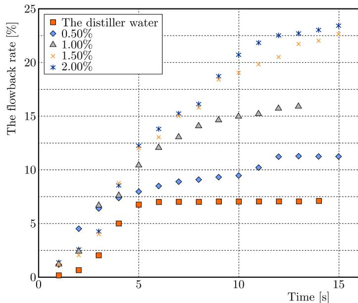
Fig. 5. The effect of interfacial tension on the backflow rate of the fluid
