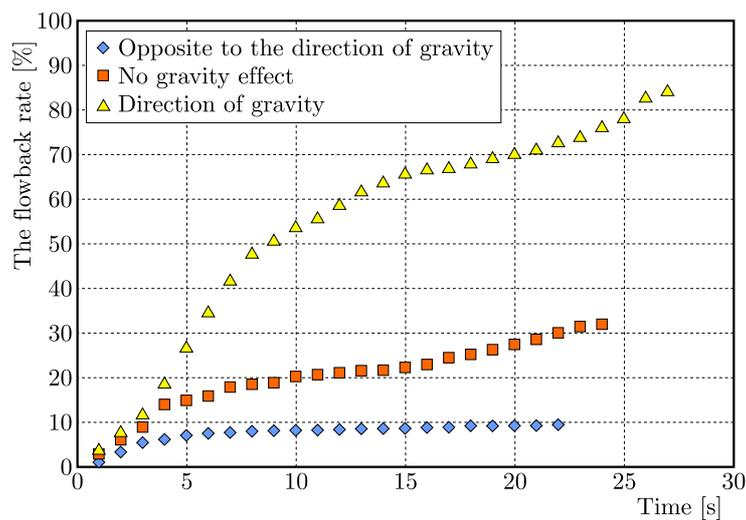
Fig. 2. Influence of the displacement direction on the backflow rate of fluid
