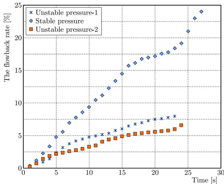
Fig. 4. The influence of pressure stability on the backflow rate
