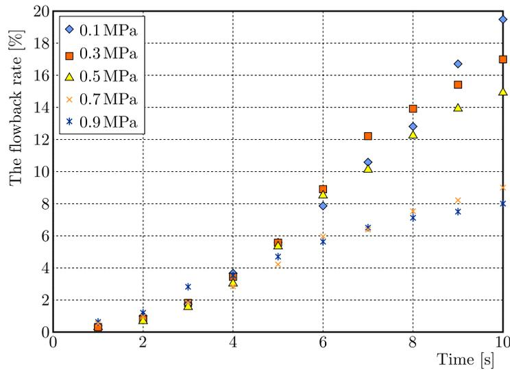
Fig. 3. Influence of injection pressure on the backflow rate
