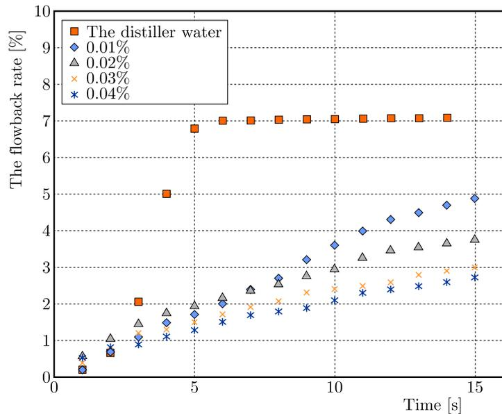
Fig. 6. The effect of viscosity on the backflow rate of the fluid
