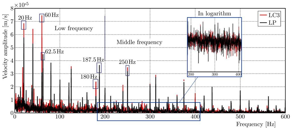
Fig. 5. A comparative analysis of the frequency response of LC3 and LP composite materials
