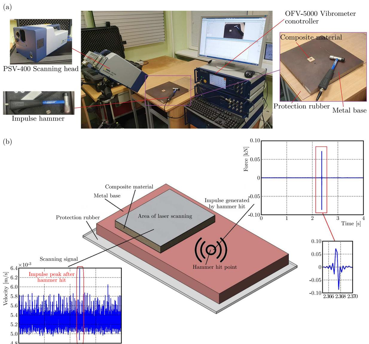
Fig. 3. Experimental details: (a) test bench for experimental measurements, (b) scheme for measurement setup
