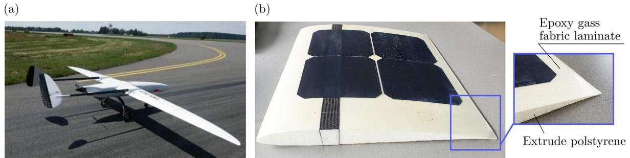
Fig. 1. The application of extruded polystyrene to unmanned aerial vehicles: (a) fixed-wing UAV (Sekar *et al.*, 2020), (b) composite structure of the wing
