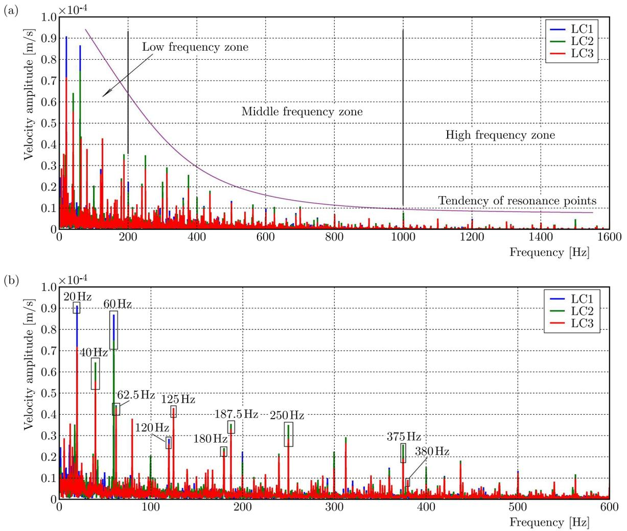
Fig. 4. The analysed spectrum of composite cork: (a) frequency response of up to 1.6 kHz, (b) frequency response of up to 600 Hz
