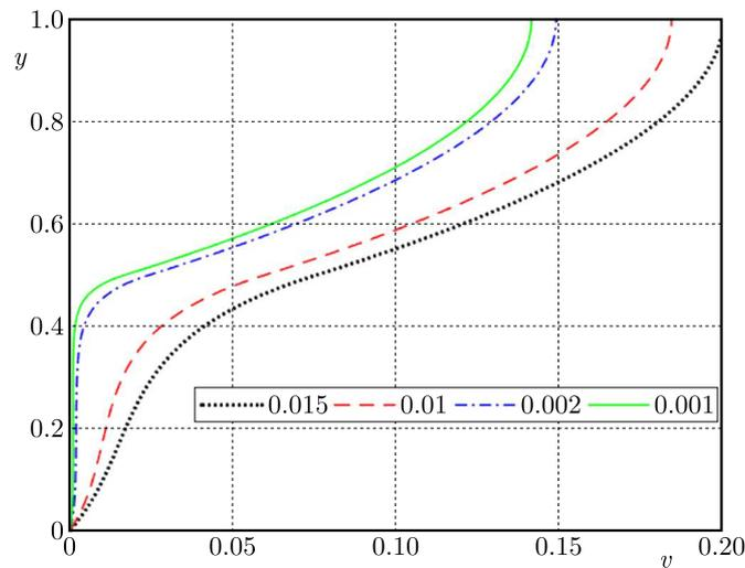
Fig. 2. Dependence of the fluid velocity  $v$  on the height  $y$  for growing permeabilities  $\kappa$  equal respectively to 0.001, 0.002, 0.010, and 0.015 (in natural units). In this case, we accept  $\kappa = \kappa'$
