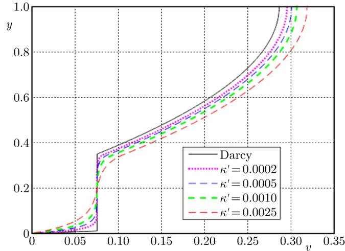
Fig. 4. Dependence of the fluid velocity  $v$  on the height  $y$  for a given permeability  $\kappa = 0.075$  and for different effective permeabilities  $\kappa'$  equal to 0.0002, 0.0005, 0.001 and 0.0025 (in natural units). The behaviour of velocity given by Darcy's equation, cf. Table 1, is given by the continuous line
