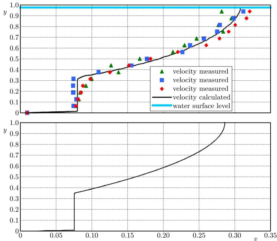
Fig. 3. Comparison of experimental results and the solution given by Kubrak *et al.* (2013) (upper) with description obtained by Darcy's law (lower). The velocity scale on horizontal axes in both figures are the same
