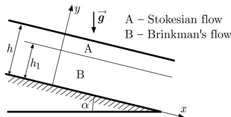
Fig. 1. Flow of the stream is developing in two manners depending on which regions of A or B, is occupied. In region A the flow is laminar, while in region B we deal with a seepage through the porous medium. The gravity acceleration vector  $\vec{g}$  has two components  $[g_x, g_y] = [g \sin \alpha, -g \cos \alpha]$
