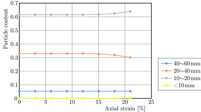
Fig. 8. Changes in the particle content of different grain size during the loading procedure
