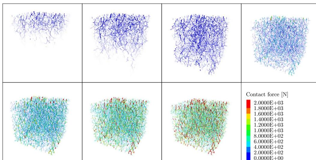
Fig. 10. Evolution law of the force chain network of gangue models
