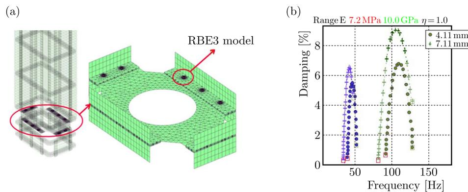
Fig. 11. Assembly with multiple bolted joints: (a) FEM model, (b) evolution of modal damping for two values of washer radius
