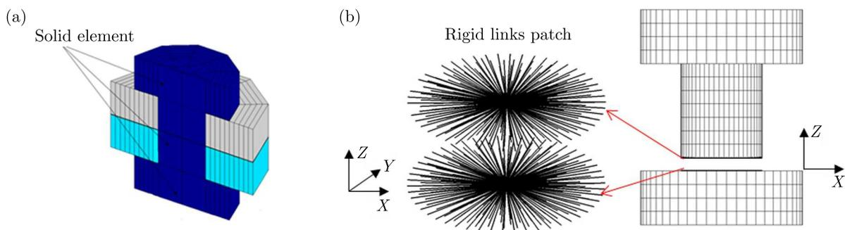
Fig. 3. Solid model: (a) finite element modelization, (b) application of the tensile force in the bolt modeled by solid elements
