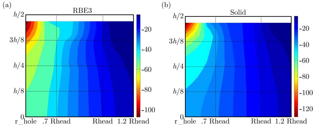
Fig. 7. Normal stress evolution in the assembly thickness: (a) RBE3 model, (b) Solid model
