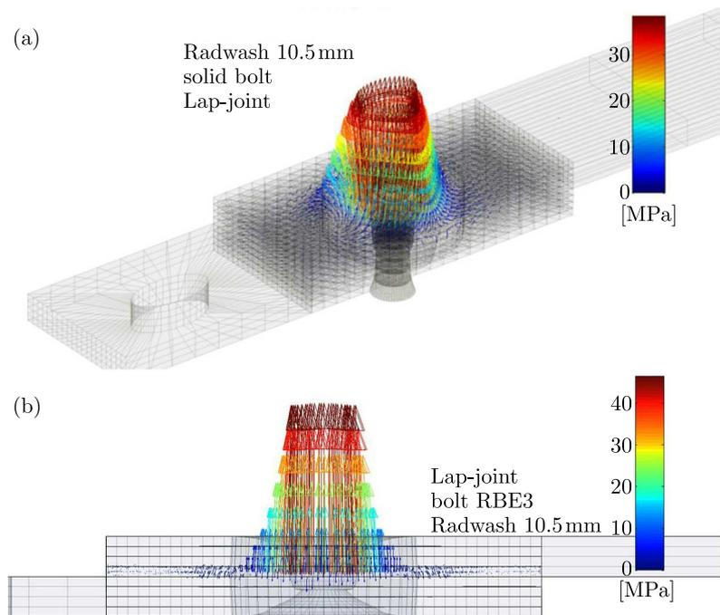
Fig. 5. Normal stress distribution: (a) solid model, (b) RBE3 model
