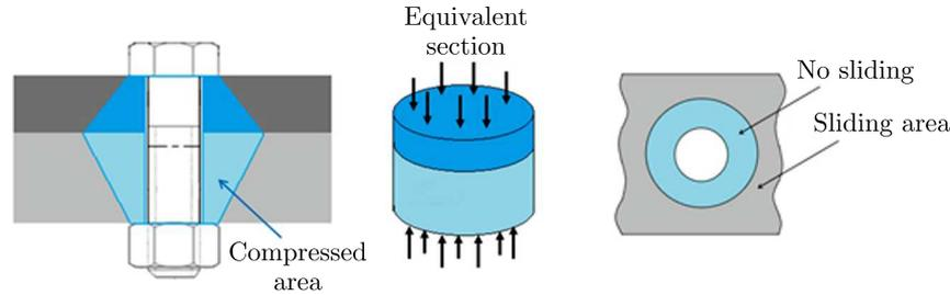
Fig. 2. Compressed area of the assembled part in bolted joints and the equivalent section
