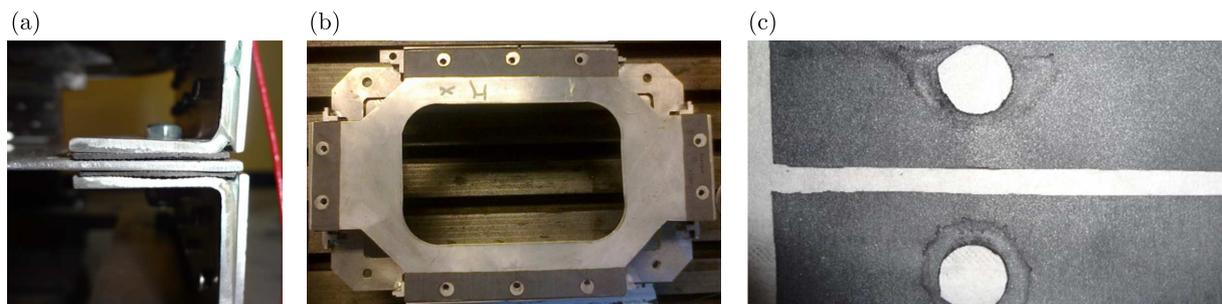
Fig. 9. Experimental test: (a) bolted joint, (b) bolted joints interfaces, (c) pressure areas in bolted joints
