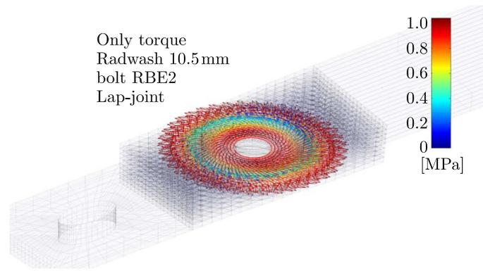
Fig. 8. Distribution of shear stresses on the interface of contact
