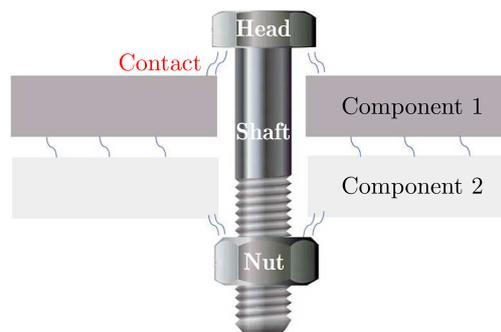
Fig. 1. Bolted joint model
