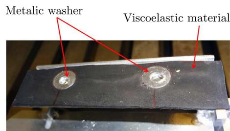
Fig. 10. Introduction of a metallic washer in the bolted joint with a viscoelastic material
