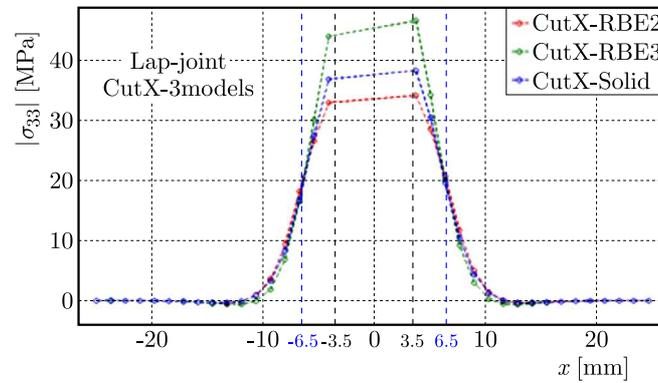
Fig. 6. Normal stress evolution on the contact interface for the Solid model, RBE3 model and RBE2 model
