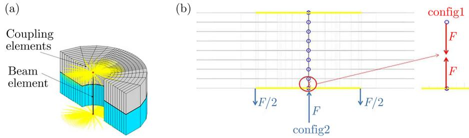
Fig. 4. RBE3 model: (a) finite element modelization, (b) application of the compressive force in the RBE3 model with beam elements
