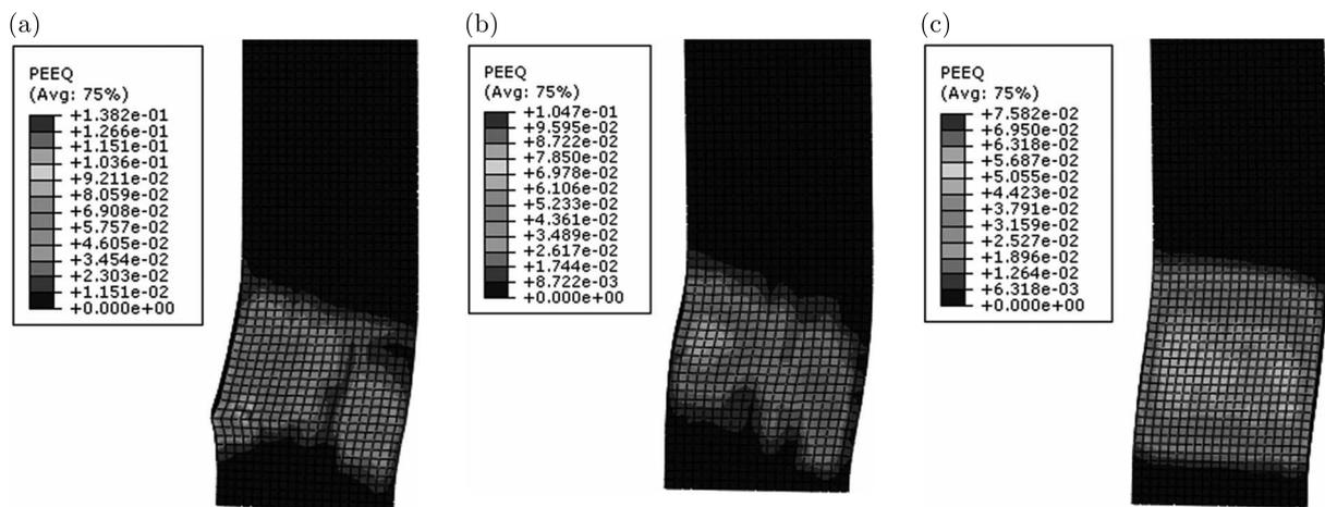
Fig. 5. Distribution of the equivalent plastic strain for pier concrete: (a) Case 1, (b) Case 2, (c) Case 3
