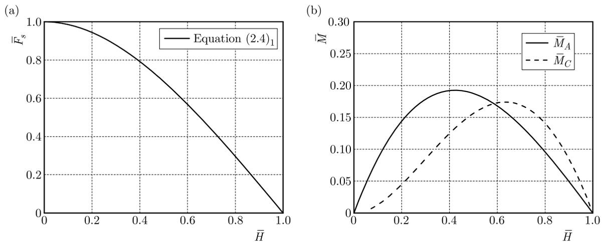
Fig. 2. Variation of (a) shear force and (b) moment with the height of loading spot
