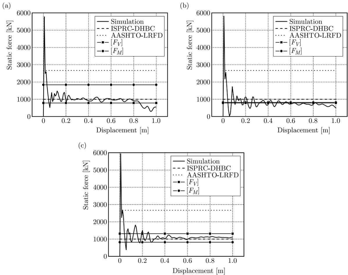
Fig. 4. Simulated lateral forces and the predicted load capacity at the loading point: (a) Case 1, (b) Case 2, (c) Case 3
