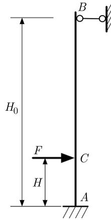
Fig. 1. The simplified beam model impacted by a concentrated load
