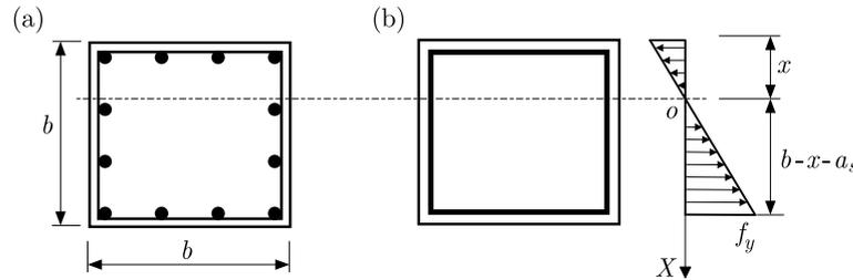
Fig. 3. Equivalent distribution of longitudinal reinforcements
