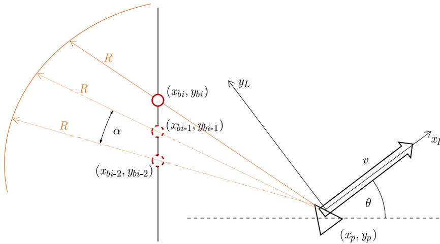
Fig. 2. Scheme of obstacle points determination
