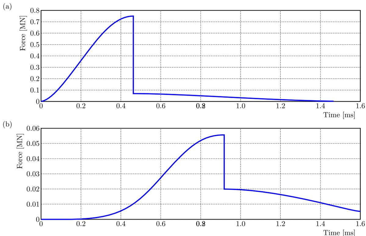
Fig. 4. Exemplary values of the collision forces in time for  $b = 110$  mm,  $m_0^r = 5$  kg; (a) collision force between feed and hammer, (b) collision force between hammer and rotor
