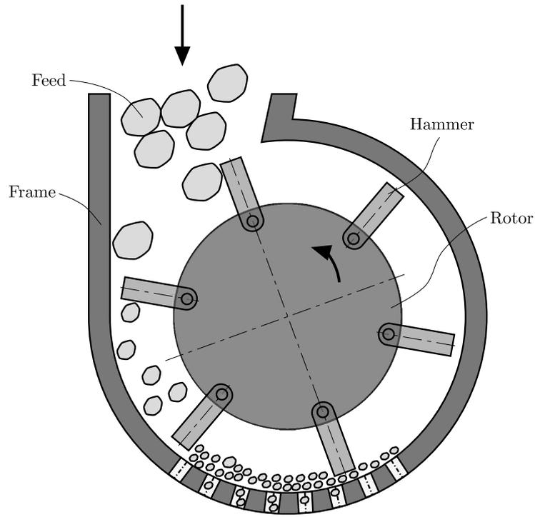
Fig. 2. A schematic drawing of the analysed hammer crusher
