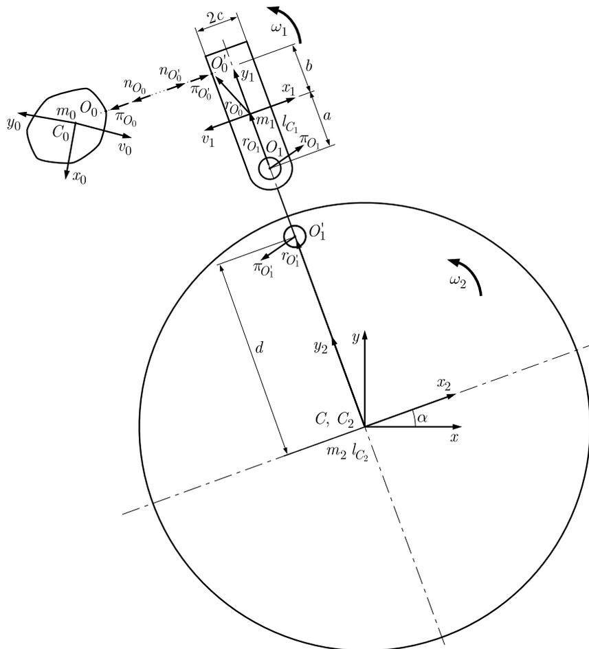
Fig. 3. Analysed hammer crusher – applied coordinates systems, geometrical parameters and kinematic quantities
