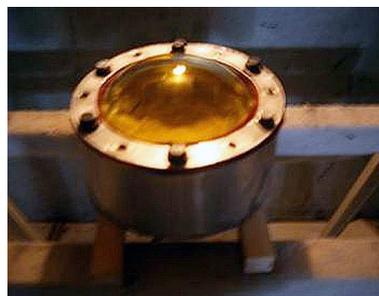
Fig. 8. Deformed plate during free thermoforming
