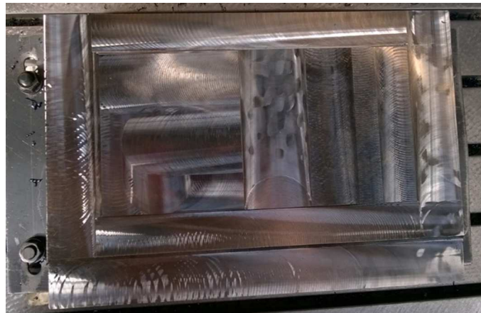
Fig. 2. View of the machined surface with marks of strong self-excited vibrations
