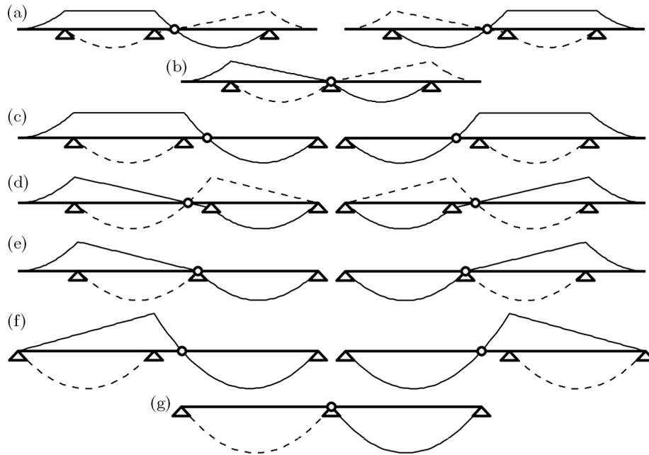
Fig. 6. All three-support topological classes with their optimal envelopes of moment diagrams: (a)  $\mathbf{T}_1^3$ , (b)  $\mathbf{T}_2^3$ , (c)  $\mathbf{T}_3^3$ , (d)  $\mathbf{T}_4^3$ , (e)  $\mathbf{T}_5^3$ , (f)  $\mathbf{T}_6^3$ , (g)  $\mathbf{T}_7^3$
