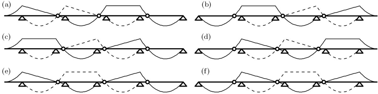
Fig. 5. All optimal envelopes of moment diagrams in the class  $\mathbf{T}_{10}^5$ : (a)-(d)  $c_{E,10}^5 = 1$ ,  $c_{H,10}^5 = 3$ ,  $c_{S,10}^5 = 2$ ,  $c_{T,10}^5 = 0$ , (e)-(f)  $c_{E,10}^5 = 1$ ,  $c_{H,10}^5 = 3$ ,  $c_{S,10}^5 = 0$ ,  $c_{T,10}^5 = 1$
