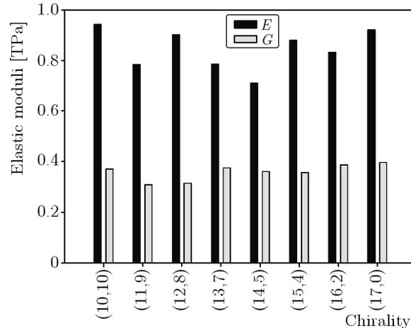
Fig. 13. The elastic moduli versus chirality for ESWCNT with the same diameter and  $a/b = 1.5$
