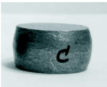
Fig. 4. leady cylinder after deformation by "Barrel Compression Test" for measurement of the friction coefficient
