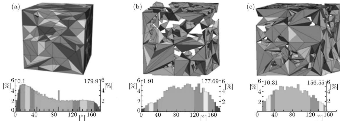
Fig. 11. Mesh quality improvement for RAND2 with two algorithms; (a) initial mesh, (b) optimized after Freitag's algorithm, (c) optimized after proposed algorithm
