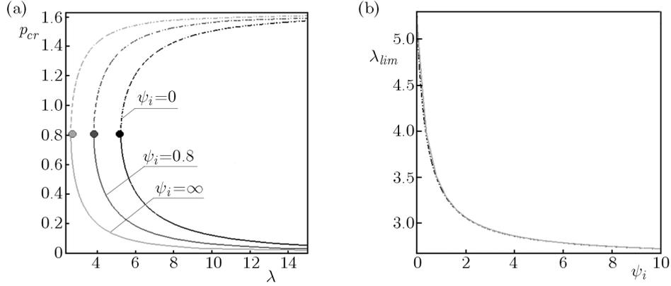
Fig. 3. Critical force vs. slenderness ratio (a), limiting slenderness ratio vs. rotational compliance  $\psi_i$  for  $\nu = 0.3$  and  $\psi_3 = \infty$
