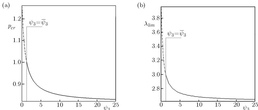
Fig. 7. Critical force (a), limiting slenderness ratio (b) vs. compliance  $\psi_3$  for the return points,  $\nu = 0.3$ ,  $d = 0$
