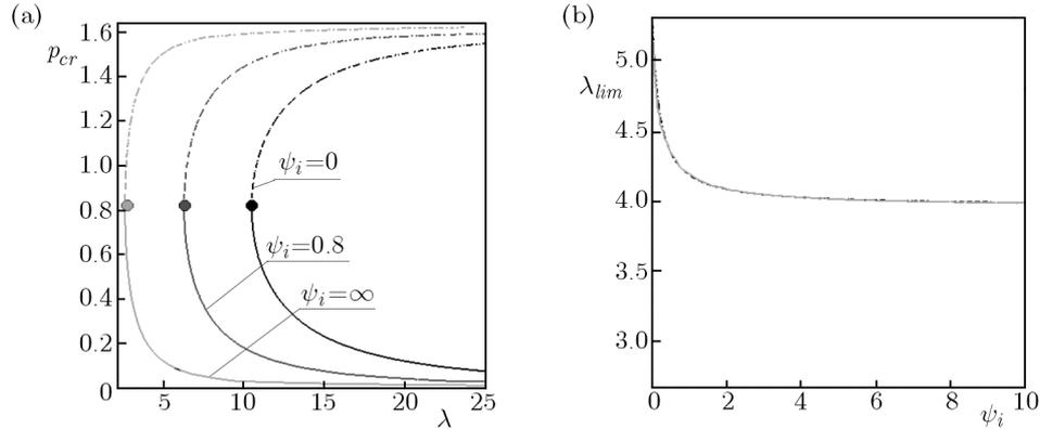
Fig. 4. Critical force vs. slenderness ratio (a), limiting slenderness ratio vs. rotational compliance  $\psi_i$  for  $\nu = 0.3$  and  $\psi_3 = 0$  (b)
