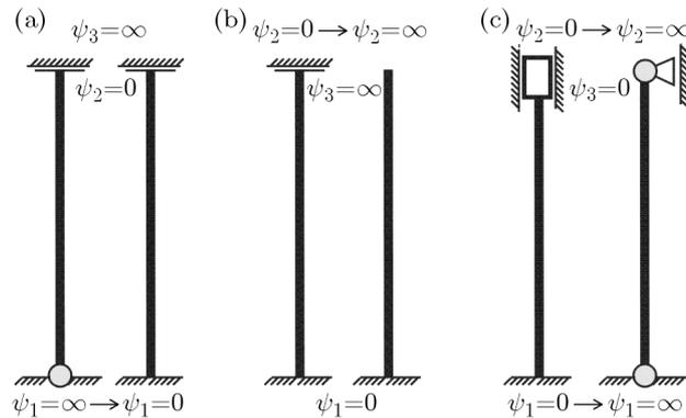
Fig. 2. Particular cases of the supports for analysis of the influence of  $\psi_1$  or  $\psi_2$
