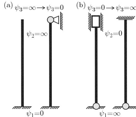
Fig. 5. Particular cases of the supports for analysis of the influence of  $\psi_3$
