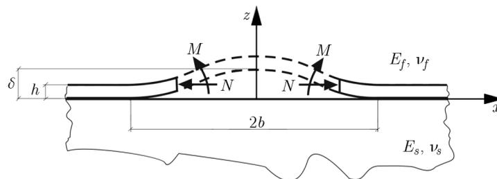
Fig. 2. Geometry and tractions for a straight-sided blister
