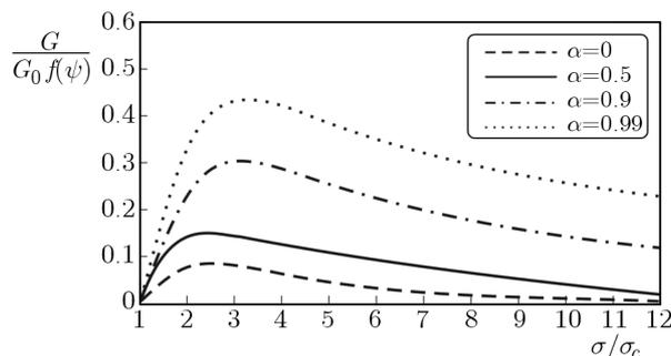
Fig. 5. The influence of differences between elastic characteristics of the coating and the substrate on the average energy release rate at the front of the blister for different values of the parameter  $\alpha$
