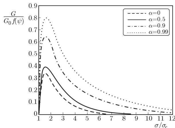
Fig. 4. The influence of differences between elastic characteristics of the coating and the substrate on the energy release rate along sides of the blister for different values of the parameter  $\alpha$
