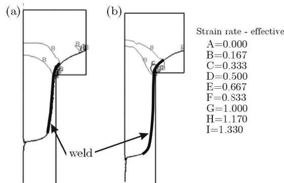
Fig. 15. Strain rates for the end of weld creation while forward extrusion through a rectangular die with a spherical face of upper billet: (a) welding with  $m = 0.4$  at the billets interface, (b) welding with  $m = 0.9$
