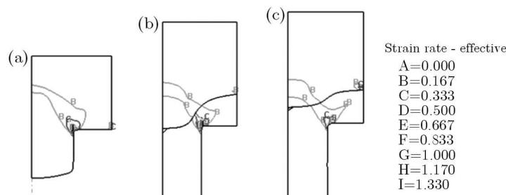
Fig. 14. Strain rates for the beginning of weld creation while forward extrusion through a rectangular die with a spherical face of the upper billet: (a) extrusion of a single billet, (b) welding with  $m = 0.4$  at the billets interface, (c) welding with  $m = 0.9$
