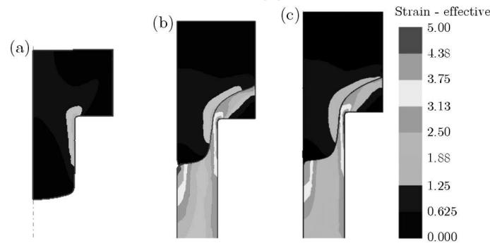
Fig. 16. Effective strain distributions during forward extrusion through a rectangular die with a spherical face of the upper billet: (a) extrusion of a single billet, (b) welding with  $m = 0.4$  at the billets interface, (c) welding with  $m = 0.9$
