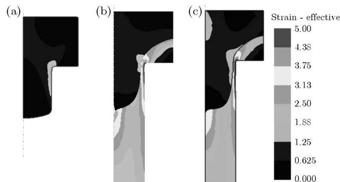
Fig. 6. Effective strain distributions during forward extrusion through a rectangular die: (a) extrusion of a single billet, (b) welding with  $m = 0.4$  at the billets interface, (c) welding with  $m = 0.9$
