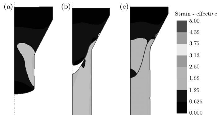
Fig. 11. Effective strain distributions during forward extrusion through a conical die: (a) extrusion of a single billet, (b) welding with  $m = 0.4$  at the billets interface, (c) welding with  $m = 0.9$
