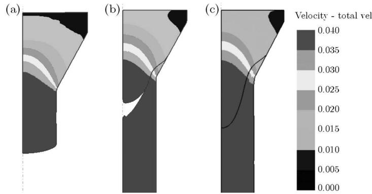
Fig. 12. Velocity distributions during forward extrusion through a conical die: (a) extrusion of a single billet, (b) welding with  $m = 0.4$  at the billets interface, (c) welding with  $m = 0.9$
