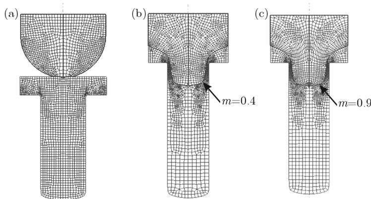
Fig. 13. Joining during forward extrusion through a rectangular die with a spherical face of the upper billet: (a) view of the billets before joining, (b) welding with  $m = 0.4$  at the billets interface, (c) welding with  $m = 0.9$
