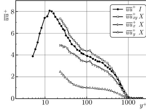
Fig. 3. The comparison of fluctuating components from single and X-wire probes
