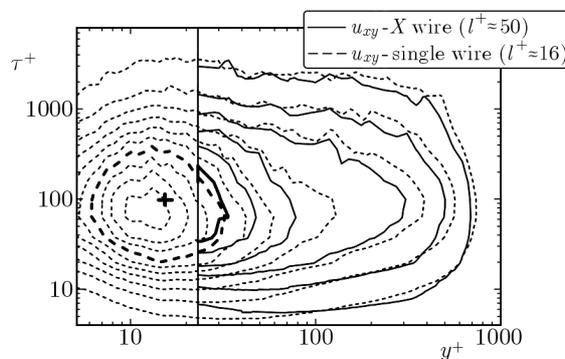
Fig. 5. Iso-contours of the energy spectra  $E(u_{xy}) = (E(u)^2 + E(v)^2)^{1/2}$  component across the boundary layer thickness – effect of the probe: X-wire  $l^+ = 50$  (solid); single-wire  $l^+ = 16$  (dashed). Contours are from 0 to 2 with the steps equal 0.2
