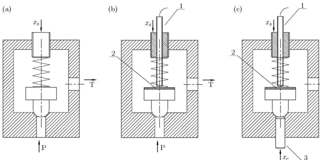
Fig. 2. Method of measuring displacements of the moving element: (a) simplified relief valve diagram; (b) fiberoptic testing probe 1 and mirror 2 installed in the relief valve for the displacement measurements; (c) relief valve, equipped with fiberoptic testing probe 1, mirror 2 and calibrating probe 3, during calibration
