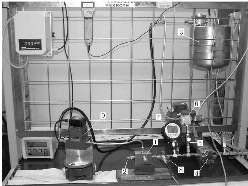
Fig. 6. The hydraulic system for measurements of the micro valve closing element displacements
