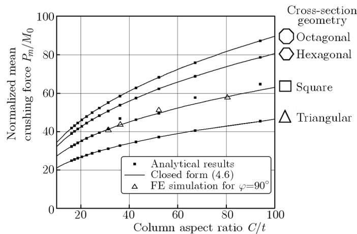
Fig. 5. Evolution of the normalized mean crushing force  $P_m/M_0$ , in terms of the aspect ratio  $C/t$  and for various cross-sections of coin elements
