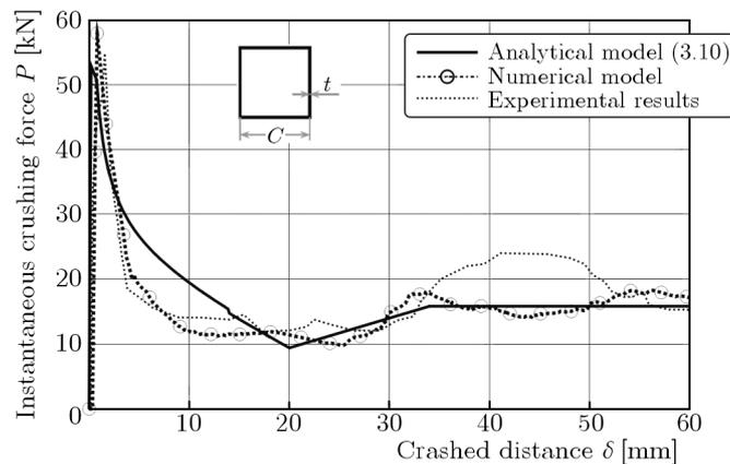
Fig. 4. Evolution of the instantaneous crushing force  $P(\delta)$  for a square column using the analytical and numerical model and compared to the experimental results from Drazetic *et al.* (1995)
