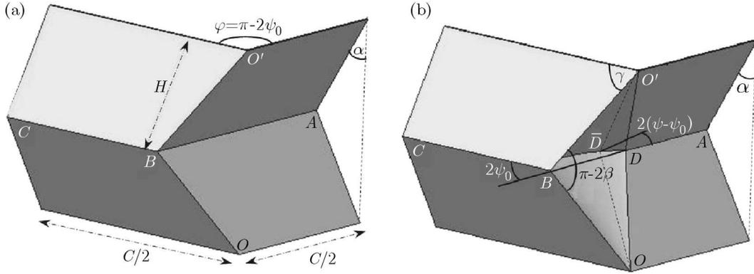
Fig. 3. Generalized mixed model; (a) phase I quasi inextensional, (b) phase II extensional
