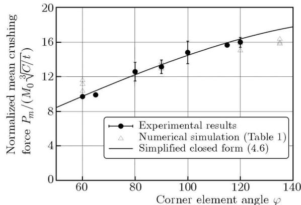
Fig. 7. Evolution of the normalized mean crushing force  $P_m/(M_0 \sqrt[3]{C/t})$  as function of the corner element angle  $\varphi$  using simplified closed formula (4.6) and compared to numerical simulation (Table 1) and experimental results from Abramowicz and Jones (1984) and Abramowicz and Wierzbicki (1989)
