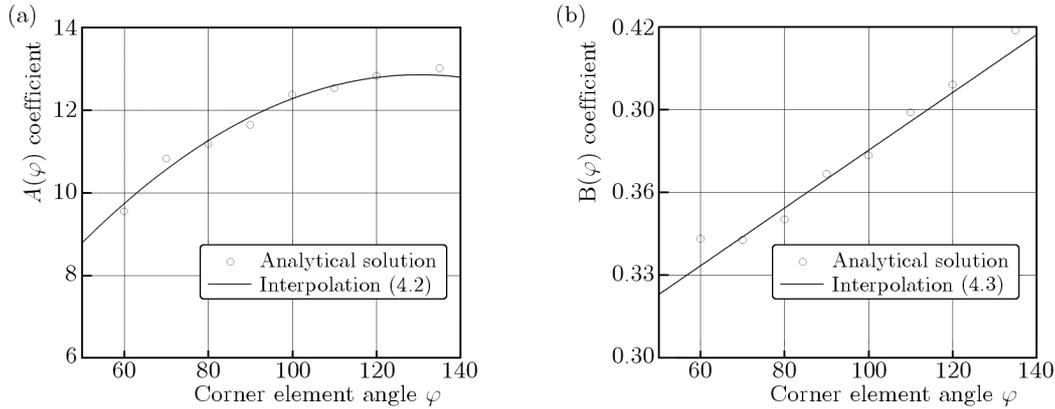
Fig. 6. Evolution of (a) coefficient  $A(\varphi)$  and (b) exponent  $B(\varphi)$  versus corner element angle  $\varphi$
