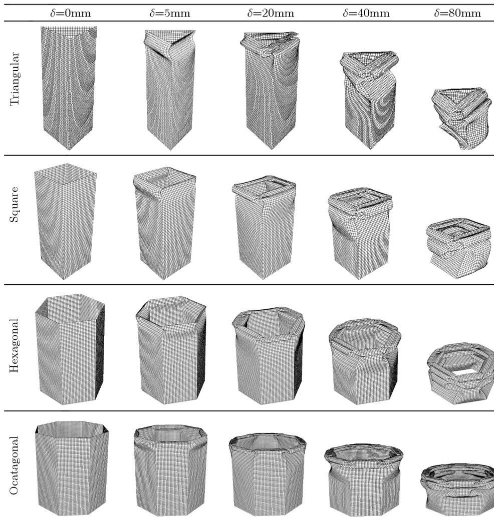
Fig. 2. Collapse modes versus crush distance for columns of triangular, square, hexagonal and octagonal cross-section geometry
