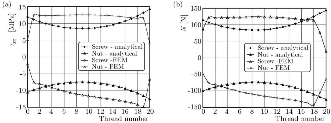
Fig. 5. Share stress distribution (a) and load distribution (b) – consistent load of the screw and nut
