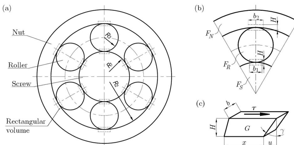
Fig. 2. (a) Model of planetary roller screw; (b) location and dimensions of the rectangular volumes; (c) load and displacement of the rectangular volume
