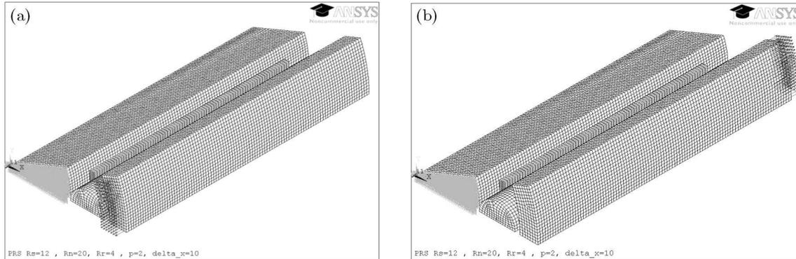
Fig. 4. FEM model of PRS – consistent load (a) and opposite load (b) of screw and nut
