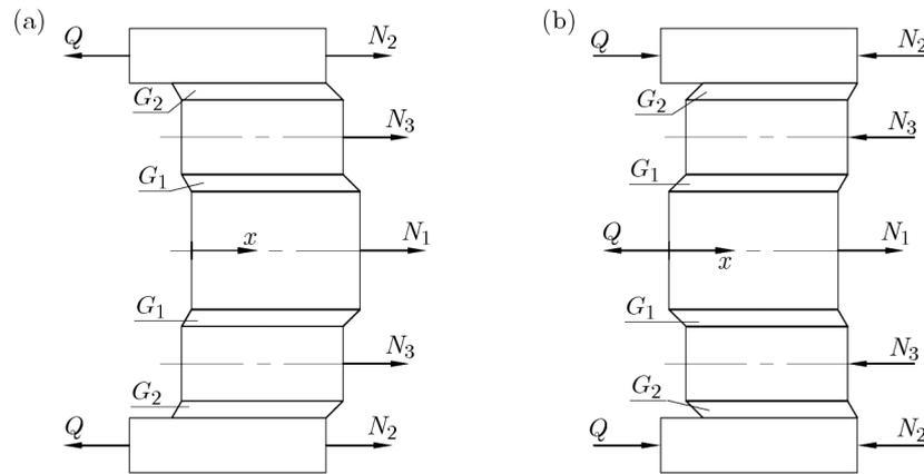
Fig. 3. Balance of forces – consistent load (a) and opposite load (b) of screw and nut
