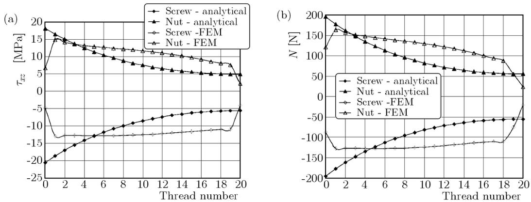
Fig. 6. Share stress distribution (a) and load distribution (b) – opposite load of the screw and nut
