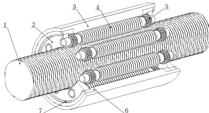
Fig. 1. Planetary roller screw; 1 – main screw, 2 – end plate, 3 – nut, 4 – roller, 5 – satellite toothed wheel, 6 – sun toothed wheel, 7 – retaining ring
