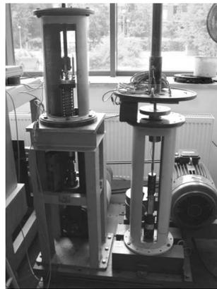
Fig. 3. Laboratory stand for investigations of VPP dampers
