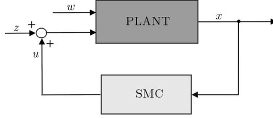
Fig. 1. Block diagram of a continuous SMC
