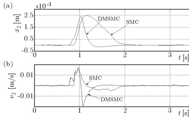
Fig. 10. Response to the impulse excitation – regulators: SMC ( $\beta_x = \beta_v = 1$ ,  $\gamma = 0.1$ ) and DMSMC ( $\beta_x = \beta_v = 1$ ,  $\gamma = 0.001$ ): (a) displacements, (b) velocities
