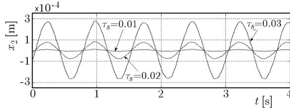
Fig. 7. Relation between the sampling time and displacements – DMSMC ( $\beta_x = \beta_v = 1$ ,  $\gamma = 0.001$ )
