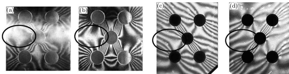
Fig. 13. Moiré pattern for model V ( $s = 0.778$ ) – grid affixed according to the direction of tension: (a)  $u(x, y)$ , (b)  $v(x, y)$ ; grid rotated by an angle of  $45^\circ$ : (c) clockwise, (d) counter-clockwise
