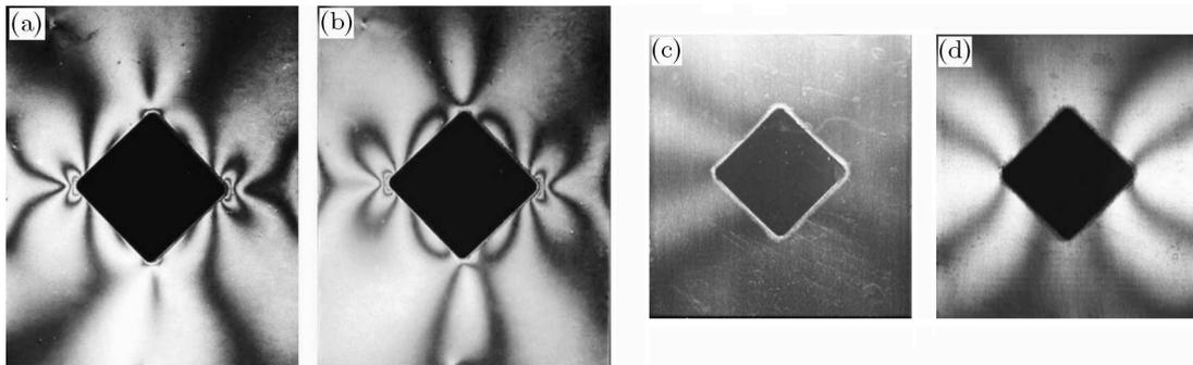
Fig. 3. Model III ( $s = 0.495$ ) – isochromatic pattern: (a) dark-field polariscope, (b) light-field polariscope; Moiré fringe pattern: (c)  $u(x, y)$  surface, (d)  $v(x, y)$  surface
