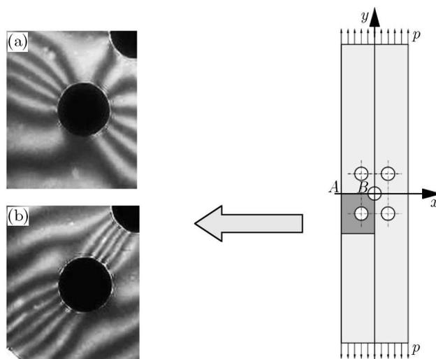
Fig. 14. Moiré pattern for the analyzed area of model V ( $s = 0.778$ ) – grid rotated by an angle of  $45^\circ$ :
