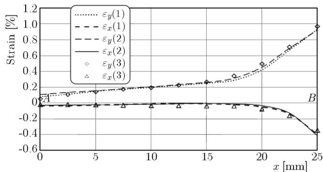
Fig. 9. Strain components distribution in the axis of symmetry  $x$  for model III –  $s = 0.952$ : (1) Moiré method, (2) method of photoelastic coating, (3) FEM calculations
