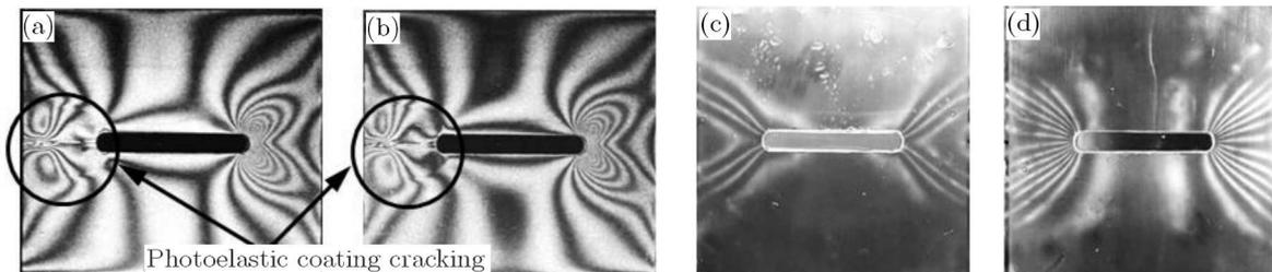
Fig. 4. Model II ( $s = 1.136$ ) – isochromatic pattern: (a) dark-field polariscope, (b) light-field polariscope; Moiré fringe pattern: (c)  $u(x, y)$  surface, (d)  $v(x, y)$  surface
