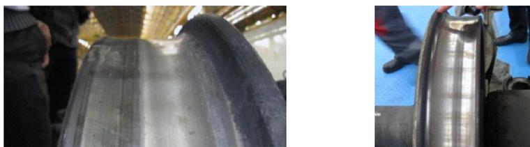
Fig. 1. Tread defects after 10 000 km passage
