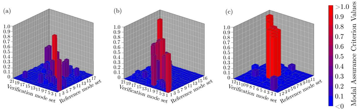
Fig. 10. Comparison of mode shapes for EMA and NMA results in terms of the Modal Assurance Criteria plot
