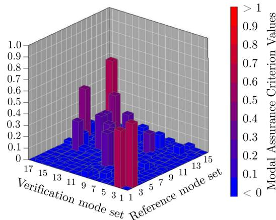
Fig. 11. Modal Assurance Criteria plot for Duct 2 with free-free boundary condition
