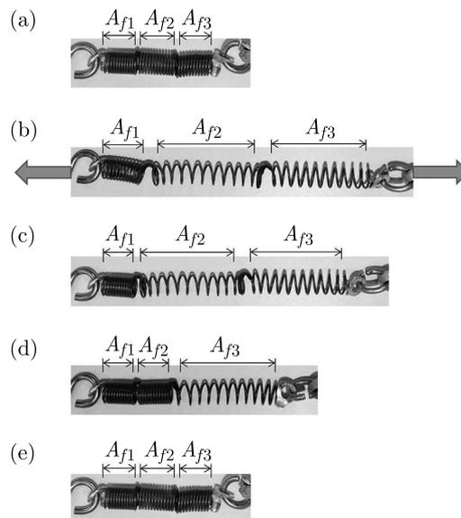
Fig. 5. Movement of the SMA coil having different transformation temperatures;  $A_{f1} = 293 \text{ K}$ ,  $A_{f2} = 318 \text{ K}$  and  $A_{f3} = 338 \text{ K}$ : (a) initial state, (b) loading at  $T = 298 \text{ K}$  ( $A_{f1} < T < A_{f2} < A_{f3}$ ), (c) unloading at  $T = 298 \text{ K}$  ( $A_{f1} < T < A_{f2} < A_{f3}$ ), (d) heating up to  $T = 328 \text{ K}$  ( $A_{f1} < A_{f2} < T < A_{f3}$ ), (e) heating up to  $T = 348 \text{ K}$  ( $A_{f1} < A_{f2} < A_{f3} < T$ )
