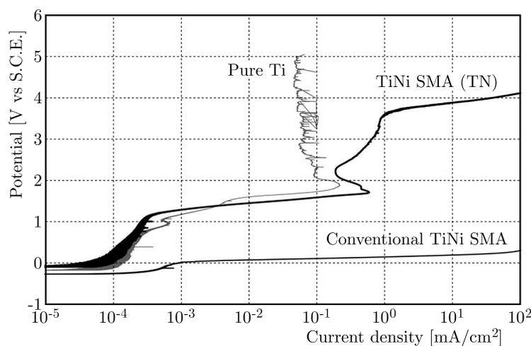
Fig. 4. Anodic polarization curves for TiNi SMA (TN), conventional TiNi SMA and pure Ti
