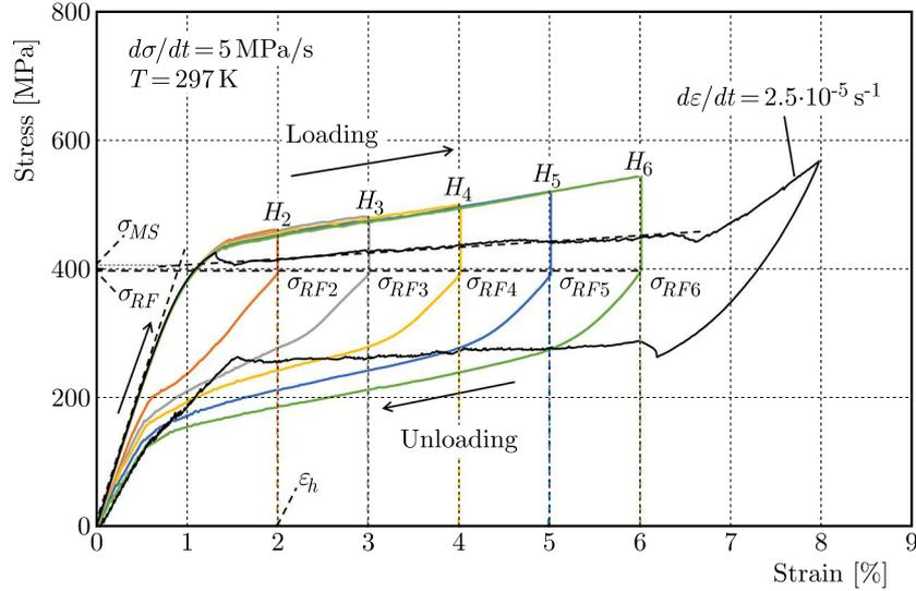
Fig. 1. Stress-strain curves of the TiNi SMA in the stress relaxation test with various holding strains and in the low strain rate  $d\varepsilon/dt = 2.5 \cdot 10^{-5} \text{ s}^{-1}$
