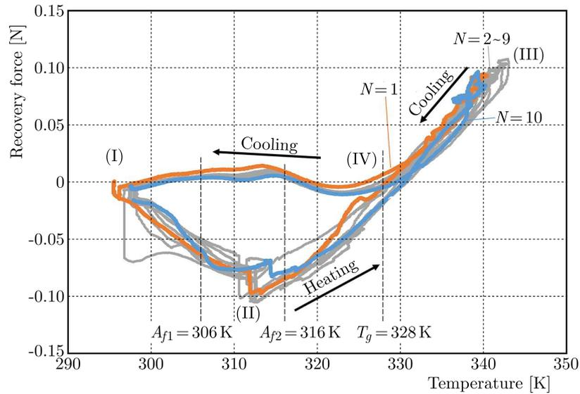
Fig. 9. Variation in the recovery force of the SMC belt during cyclic heating and cooling
