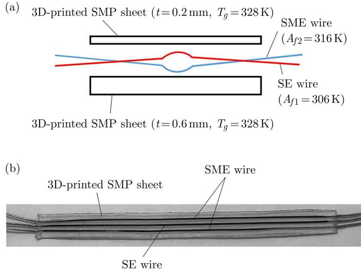
Fig. 8. Structure (a) and photograph (b) of the SMC belt
