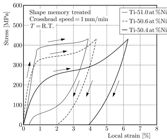
Fig. 6. Stress-local strain curves of FGSMA wire with gradually changing composition
