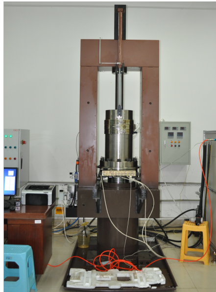
Fig. 1. TFD-2000 electro-hydraulic servo rock triaxial testing machine.
