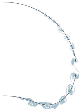
Fig. 6. Smoothed contour ( \delta = 0.1 ) in black, in front of the \delta = 0.008 interface (gray). Contours associated with the thickness at z -axis. Shifting along z applied to match the heights.
