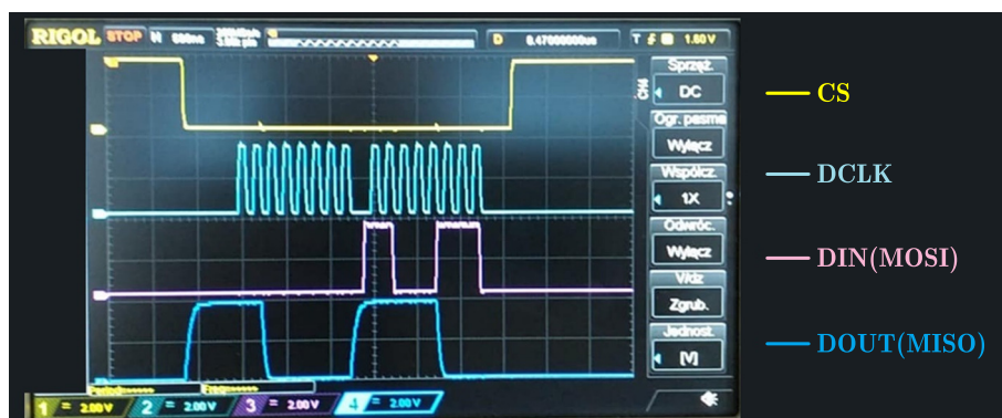
Fig. 3. Oscilloscope capture of a single SPI data exchange sequence between the microcontroller and the MEMS sensor, illustrating the timing relationship between clock and data lines.
