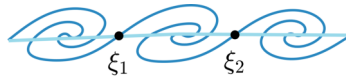
Fig. 4. Conceptual drawing of a material piece of the interface before (light) and after (dark) the roll-up. Its initial length ( \xi_2 - \xi_1 ) is a good measure of the eddy size.
