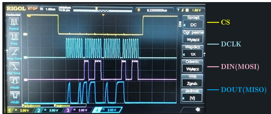
Fig. 4. Oscilloscope capture of SPI communication in reduced sampling mode (every second byte), showing selective acquisition of relevant data segments.
