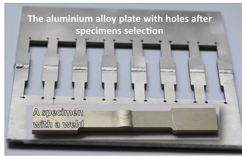
Fig. 4. Aluminium alloy plate after specimens manufacturing for examination of mechanical resistance of the weld.
