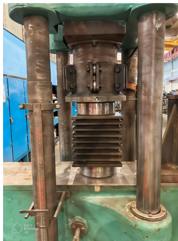
Fig. 1. Test bench set to measure spring characteristics.
