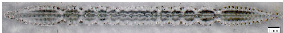
Fig. 2. Plexiglas plate after the mode shot performed with the applied laser beam.
