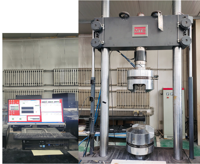
Fig. 2. MTS-793 rock mechanics testing machine.
