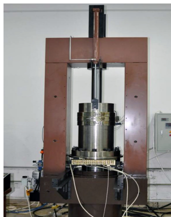
Fig. 5. TFD-2000 microcomputer servo-controlled rock triaxial testing machine.
